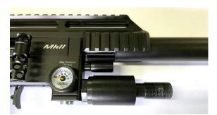
Now place the collar of the regulator on the regulator body. Make sure the blind hole with small measuring hole faces towards the same size as your factory pressure gauge. Then put the o-ring, what you removed from the bottle valve adapter, on the treaded part of the regulator
