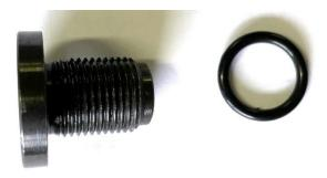
Deburr and clean the adapter afterwards and put on the thicker o-ring what is supplied with your new regulator (it is inside the facing of the regulator) and screw the adapter into the regulator body. Hand tight is sufficient.
