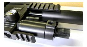
Now you can screw the bottle on the regulator body. Before you tighten the bottle, please align the regulator collar to the position you want it and after that, tighten the bottle firmly by hand. After this you can place the pressure gauge and the foster fill connection to the collar of the regulator.
