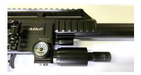
Now place the collar of the regulator on the regulator body. Make sure the blind hole with small measuring hole faces towards the same size as your factory pressure gauge.
