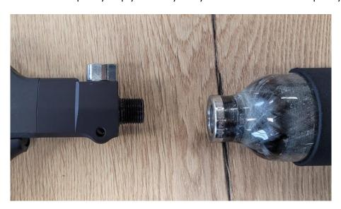
Now unscrew the bottle to reveal the screws holding the regulator holder in place.
