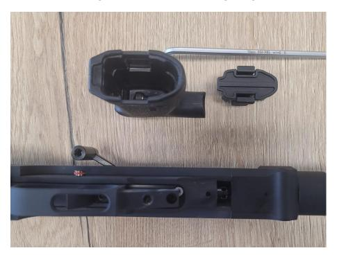
You might need to adjust hammer spring tension. To reveal the adjuster the grip needs to be taken off. To do this you will need to unscrew the M6 screw inside the grip using a 5mm hex key.
