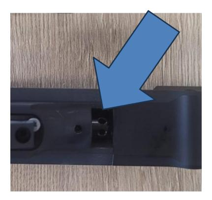
The adjuster can be found under the grip. Adjust according to  $\underline{\text{these}}$  instructions.
