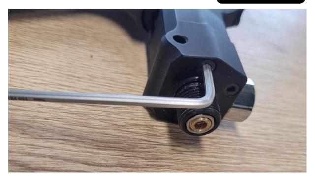
Unscrew the screws in steps unsing a 3mm allen key, and make note off the torque requires to unscrew them to give you a feel how hard they need to be tightened afterwards. When unscrewing first undo all 3 only a little in a crosswise pattern. Repeat the steps untill all 3 are loose.
