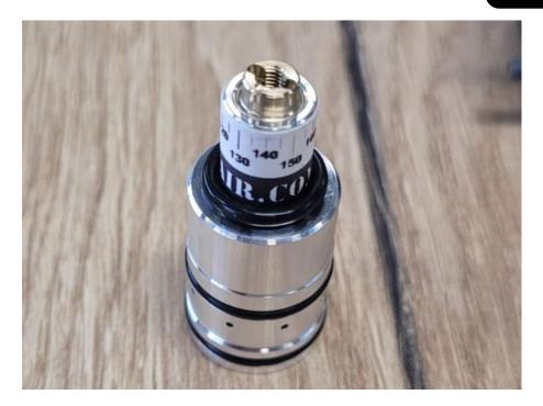
Transfer the oring that is on the small diameter part to our regulator. This will keep tension on the regulator while assembled and push it back into the regulator adaptor block.
