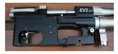
Unscrew the pressure tube from the action and after this, unscrew the original regulator from the pressure tube. It can be tight so a piece of rubber or leather belt can help you unscrew it without causing damage. After this, remove the pressure gauge assembly. In the action/regulatorbody there is the original valve return spring. Don't forget to place it back again!
