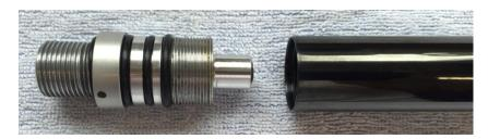
The position of front O-ring of the new Huma regulator is a few mm further inside the pressure tube compared to the original regulator.(see mark on the tube) Please check the surface of the inside of the tube were the o-ring will be seated, if it is smooth and without scratches. If not, please polish the surface of the tube until it is smooth. When finished clean the tube well and put a bit silicone grease inside the first 30-40 mm of the pressure tube.
