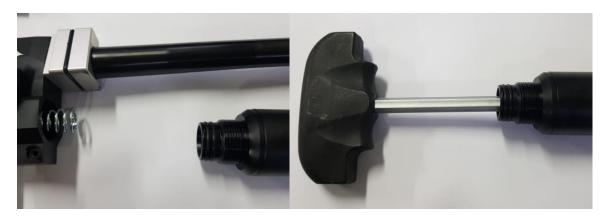
When unscrewing the cylinder from the action, most of the times the endplug will come out together with the cylinder. You can use a fitting hex wrench to unscrew the plug from the action.
