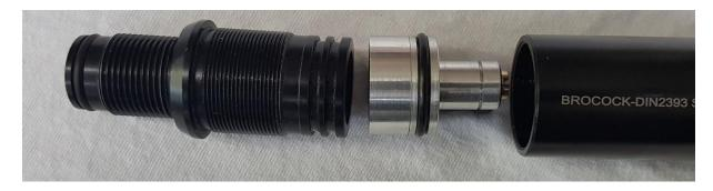
Make the treads of the tube and valvehouse clean of grease and screw it back into the pressure tube. Tighten it by hand, and after you have tighten it unscrew the valvehouse for about a quarter of a turn leaving a tiny gap between tube and adapter. This will help your regulator to breath free.
