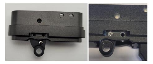
Now reinstall the pushrod back into the new triggerblade and reinsert the little pin
