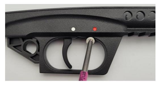
Then push the pins to one side so force to push out the pins is kept to a minimum
