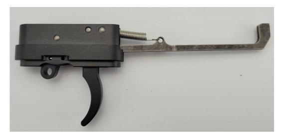
You will now insert the subassembly in the actual trigger frame. Slide it nice and straight into the triggerframe until it is flush with the bottom.
