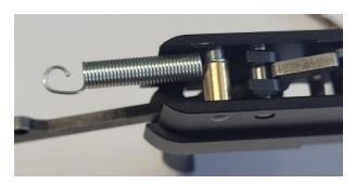
Last step is to hook the spring to the pushrod, then the subassembly is done.
