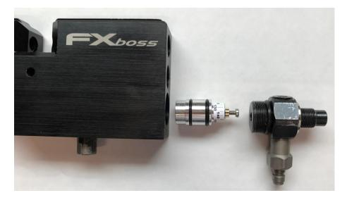
Check if the regulator is fully inserted. It should be inside the chamber for about 23 mm. (FX Boss)
