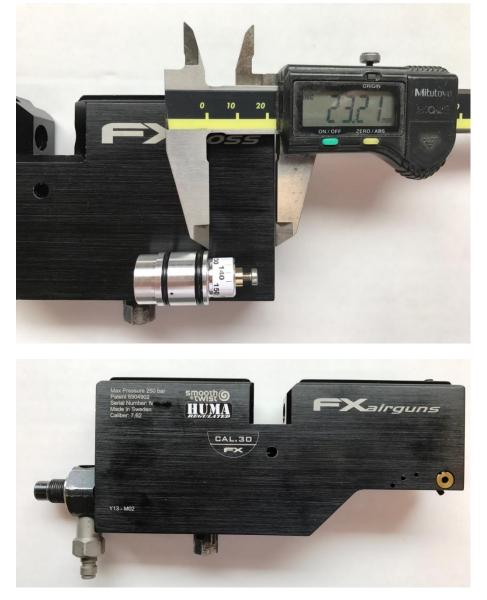
Please check if the adapter does not touches the setscrew when it is screwed in again by measuring the length. (If it does, the reg needs to be pushed into the rifle some more OR open up the hole in the bottle adapter for about 2-3 mm in length and 8 mm diameter, but this is very unlikely)
