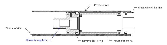
After this screw the pressure tube on the action and you can assemble the rifle back again. If you like you can stick the "Huma-Air Regulated" sticker on the action.
