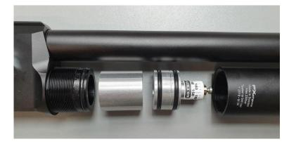
Now slide in the Huma-Air aluminum spacer, this will hold the reg in the correct position in the tube. This additional spacer of plenum will ad about 14 CC of regulated air to your rifle!
