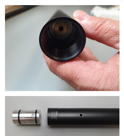
Now take the Huma-Air power tune regulator set and check if the regulator is fully clean and free of dirt. If not, clean it and apply some silicone grease on the walls of the pressure tube. Then slide the new regulator into the pressure tube, facing the label side to the barrel end.
