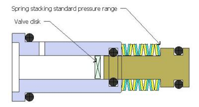
(If the max output pressure is not high enough, please ad 1 set of 2 FX factory springs to the bottom of the piston so there will be a total of 16 springs)
