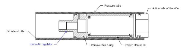
Check if the regulator is fully clean and free of dirt. If not, clean it and apply some silicone grease on the walls of the pressure tube. Then slide the new regulator into the pressure tube, facing the label side to the barrel end.
