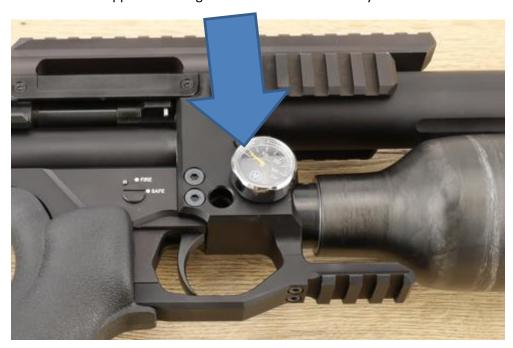
After unscrewing the gauge you can use a small pin to push out the nozzle.
