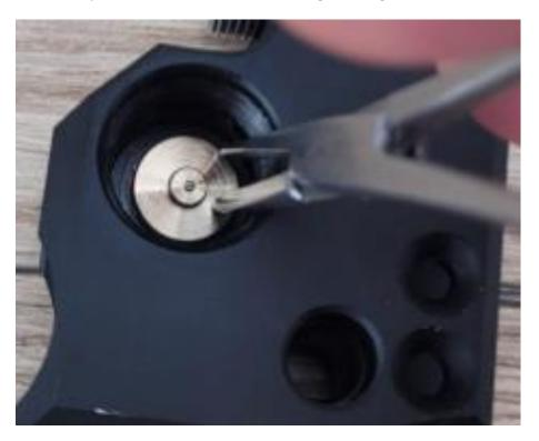
Now insert one of the valvediscs (just one) in the black regulator body with the marked face pointing upward it should stay in place by the silicone grease that is in the regulator. Note 2 valvediscs are supplied. The 2<sup>nd</sup> one is a spare in case the first one does not close accurately and you experience some creep on the oring!
