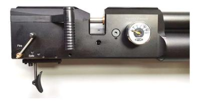
Unscrew the factory pressure gauge.
