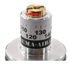
The BSA R10 models have a small dot on top of the setscrew. This dot correspondences with the position of the pressure scale.
