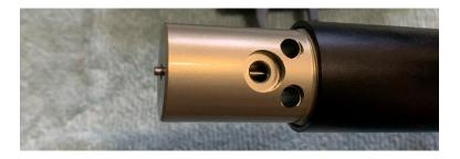
Unscrew the valve body from the pressure tube/air cylinder,
