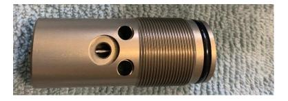
Make sure the valve body and threads are clean and free of grease and oil,
