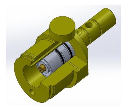
After that the OEM lock nu can bes screwd in to sequrely hold the regulator.
