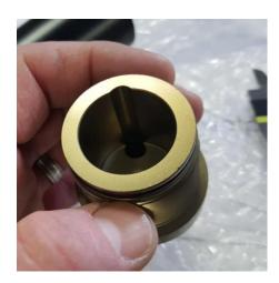
Make sure the inside of the pressure tube has no scratches or dirt inside it,
