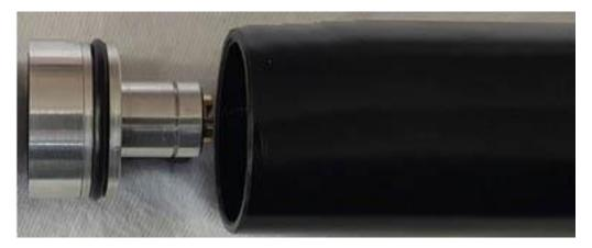
Make sure the tiny breath-hole of the regulator body is facing upwards to the breech when the tube is screwed on.
