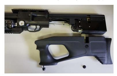
Drain the pressure tube so the rifle is totally empty by, for example, dry fireing
