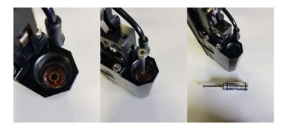
Whipe out the regulator chamber using a piece of paper towel. Now you can install the HuMa-Air regulator. Before installation apply a bit of silicone grease to the o-rings.
