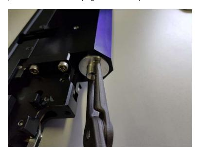
If the high pressure line is in the way you can easily remove the small cap that secures the line.
