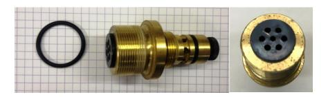
Make sure the inside of the pressure tube has no scratches or dirt inside it,
