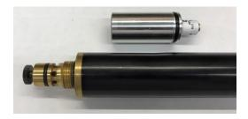
Unscrew the valve body from the pressure tube/air cylinder,
