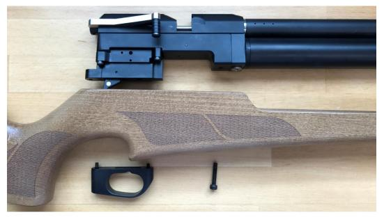
2. Remove the barrel, barrelshroud by loosing the grubscrews in the breech.
