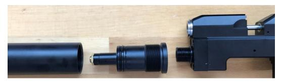
4. Unscrew the factory regulator en replace it by the Huma-Air tuning regulator
