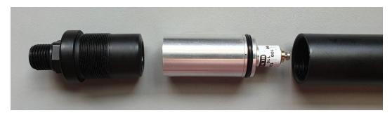
11. Now you can screw the endcap into the pressure tube again. Before you pressurize the tube again, please unscrew the pressure tube just about a ¼ to a half turn open, so there is a tiny gap (max 0,5-1 mm) between the pressure tube and the pressure tube endcap. This allows the regulator to breath to the atmosphere
