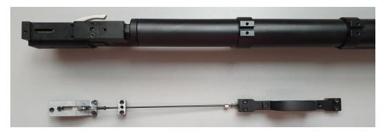
4. Loosen the two side bolts of the barrel- tube clamps
