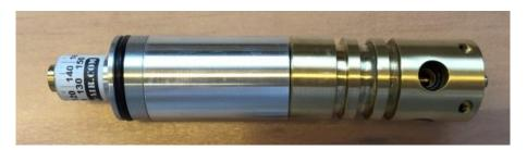
Now push the regulator-valvehouse combination into the pressure tube from the fill side. (do not try to push it in from the trigger-side, the slots in the pressure tube will damage your orings for sure)
