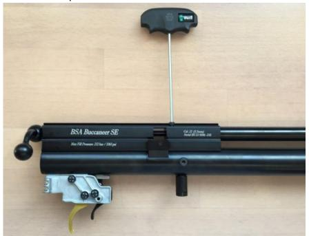
Unscrew the bottom screw what holds the breech.
