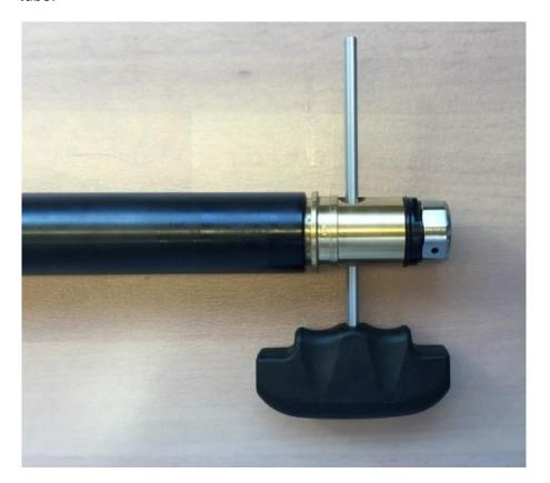
Now you can push out the valve house from the back of the rifle to the front using a rod or a piece of wood.
