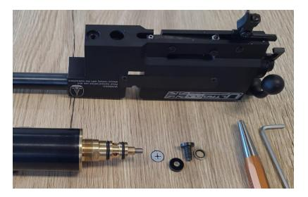
This will give you easy access to the valvehousing and you'll have the option of using the flats in case the valvehousing is tighter than our example.
