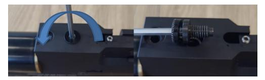
Now using a 3mm hexkey unscrew the screw. The plug will be forced out by the screw. Take note that under the screw is a bonded seal. Avoid losing that  $\mathfrak{S}$ .
