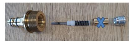
Here are the parts in succession. You will need to remove the brass restrictor. After removal of the restrictor reassemble the valve again.
