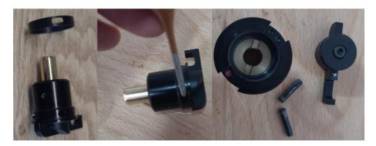
Remove the Delrin collar that covers the pins holding the safety, tap out the pins which will free the safety lever. Watch out you will not loose the small ball detent and spring.
