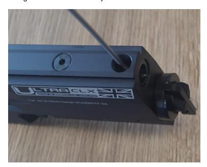
Remove the screw that holds the safety assembly. Be sure to put some pressure on it, otherwise it will come flying out of the breechblock.
