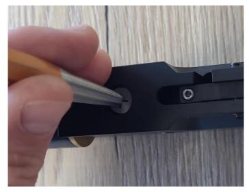
Now take a drill of around 4,5mm and drill through the aluminium plug trying to avoid marring the screw underneath. Try to avoid getting swarf in the trigger parts by masking it with a plastic bag and some tape.
