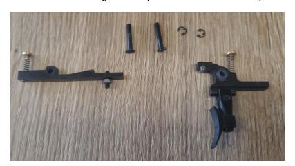
Then push out the pin making sure nothing springs from it's place. You should get the above parts out.
