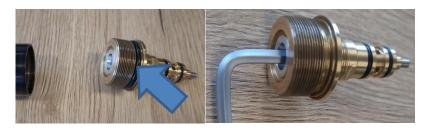
Remove the the valvehousing from the tube, remove the oring and unscrew the aluminium plug from it.
