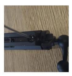
Now using a 2mm hexkey start unscrewing the screw under the plug. Due to the location of the screw being slightly off center, you might need to help the right side of the plug a little with a screwdriver. After a couple of mm you should be able to pull the plug out with a pair off needlenose pliers.
