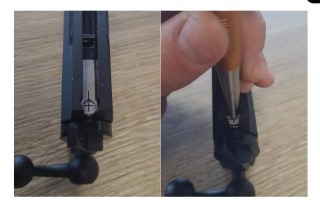
Cut out the 2<sup>nd</sup> centering help and place it on the 2<sup>nd</sup> plug. And center the slight off center place. Start with a 1mm drillbit and just drill the aluminium plug. Then follow that one with a 3mm drillbit making sure you only drill the aluminium and don't damage the hex connection of the screw underneath it.
