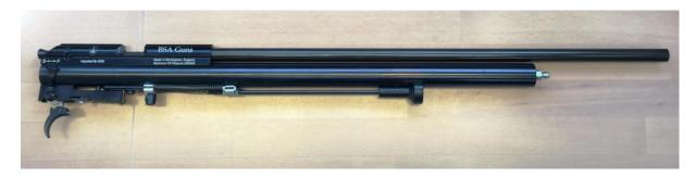
Loosen both the breech screws a bit so there is a bit space between pressure tube and breech. This prevents scratches on the tube when turning it loose.
