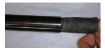
Continue with removing the outer O-ring of the valve house. You won't use it anymore, just like the restrictor and valve endcap.
