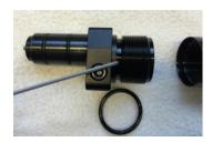
Place the regulator into the valveblock with the tiny breath hole facing in the opposite direction of the rifle's pressure gauge.
