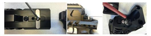
If you notice power spikes every few shots it means that the regulator is not venting/breathing enough/properly. Check that the threads of the pressure tube and valve body are clean and free of grease, also make sure the valve block is not screwed too tightly into the air cylinder.
