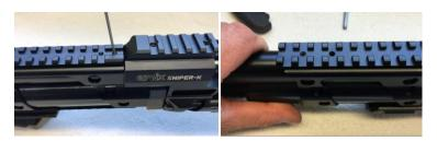
Unscrew the endcap of the fill-side and unscrew the allen bolt from the underside of the barrelband. Then carfully remove the barrelband by sliding it off. And also slide off the hand-grips.
