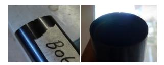
file a small groove in the longitudinal direction of the screw-thread of the valve body. Use the corner of the file to cut a 45 degree/triangular groove in the threads, as shown below,
