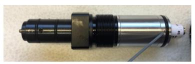
Screw the pressure tube together again and leave a tiny gap (0,5 mm) open between valveblock and pressure tube so the regulator can breathe.
