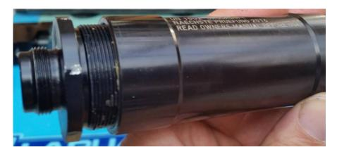
Now remove the o-ring of this endplug, optionally you can file a small groove to the thread root (direction marked in red) and in the end of the tube for the regulator to breath. (not essential)
