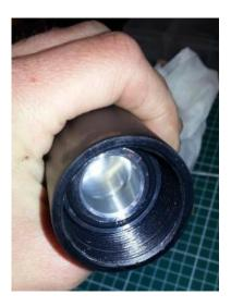
After this you can screw the endcap back on and pressurize your cylinder to check for any possible leaks.
