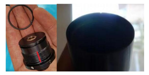
Now take your regulator and using a little silicone grease, grease your o-rings lightly. This will help in sliding in the regulator. Insert it so the face o-ring is facing the threads. So it will seal on the end plug.
