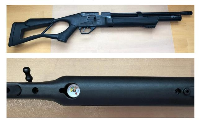
Behind the pressure gauge there is a bleed screw what allows you to drain the pressure out of the tube. You can open it up for about  $\frac{1}{4}$  to a  $\frac{1}{2}$  turn. Be careful and use safety goggles because high pressure air will escape.
