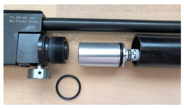
Make sure the valve body and threads are clean and free of grease and oil, and check if the inside of the pressure tube has no scratches or dirt inside. Lightly grease the first 7 cm of the pressure tube with silicone grease, (nothing else) Check if the O-ring is properly seated in the groove of the plenum/spacer of the regulator and carefully push the regulator into the pressure tube as shown in the picture below.
