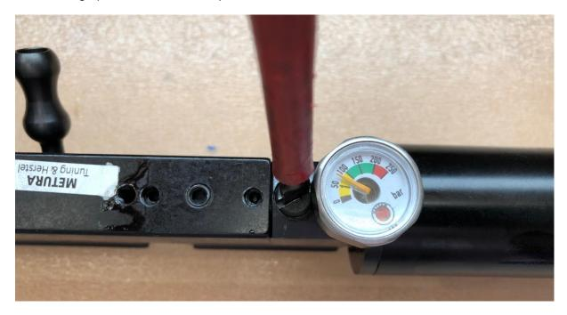
Check the air has been completely drained before you continue. Mark the upper side of the pressure tube, facing the breech side, Now remove the air stripper of the barrel and remove the barrelband
