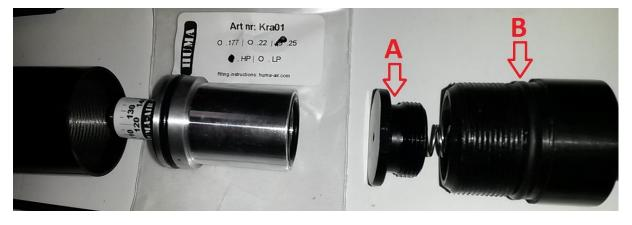
Unscrew the valvehouse cap and place the small o-ring what came with the regulator on the cap "A" Then grease the o-ring seating on the valvehouse a bit for smooth fitting. o-ring "B" has already been removed in the steps before.
