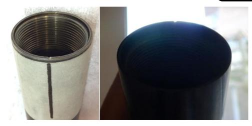
After you have done this screw the valve body into the pressure tube/air cylinder.
