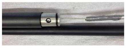
8. You receive your regulator in a small plastic bag. The bag contains the regulator and also a tiny M3 allen flow restrictor bolt that has to be placed inside the adjustment screw. This bolt creates a slower but more accurate regulating behavior.
