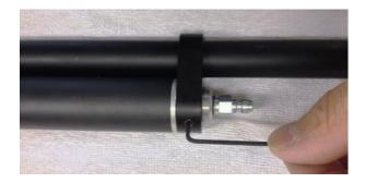
5. Take a pair of pliers to remove the end cap. Use a piece of leather (belt) to prevent damage to the end cap, and unscrew the end cap.
