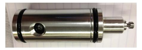
After you have removed the original pressure gauge adaptor, slide the regulator in the pressure tube. Make sure the hole of the pressure gauge is lined up with to the hole in the pressure tube!!
