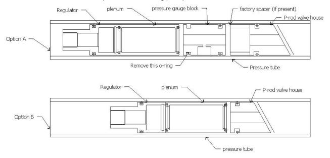
9. You can use a piece of PVC electric installation pipe to push the regulator in. Please do not push on the set screw because this can adjust the regulator pressure
