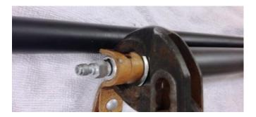
5. You should be able to push the pressure gauge assembly a little forward into the tube, using an allen wrench o wooden dowel that you place in the hole of the pressure gauge.
