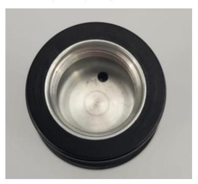
To this part place an air blower pistol used on your shop compressor and place a piece of tissue in the regulator orifice then cover it tightly with your hand. And then apply pressure.
