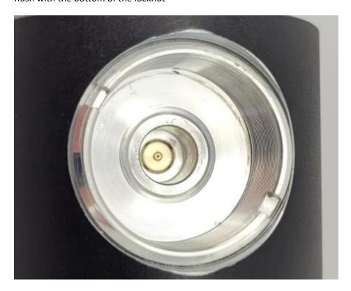
Insert the valvedisc in the bore or using a little silicone grease on the piston face "glue it on the piston" then you can commence to screw in the complete subassembly.
