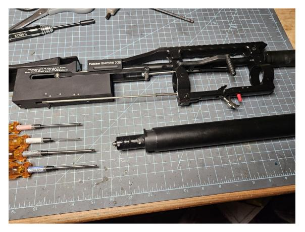
5) Once the valve/air tube have been removed, you will need to remove all the remaining pressure in the tube.
