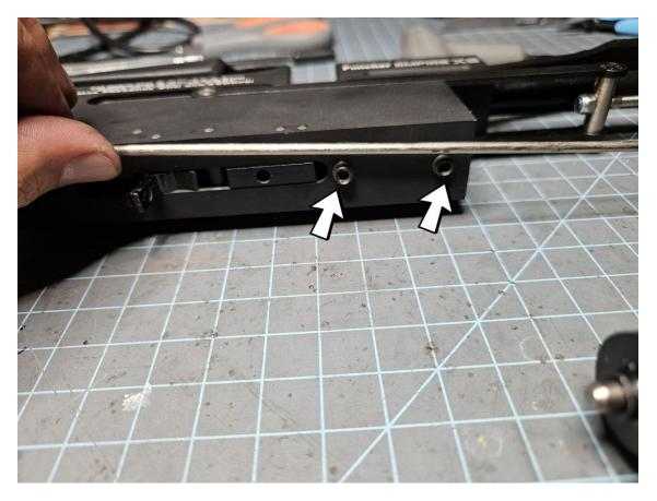
4) Remove the valve/air tube by pulling on the tube from the barrel end. A slight back and forth twisting motion will help get the valve body moving out of the receiver block. Go slow and steady to not damage the two o-rings on the valve body.
