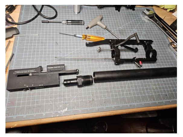
7) Remove the two o-rings from the valve body, unscrew the cap, and set aside the cap and valve spring.
