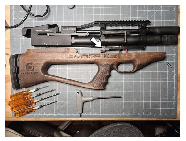
3) Loosen the valve body set screws
