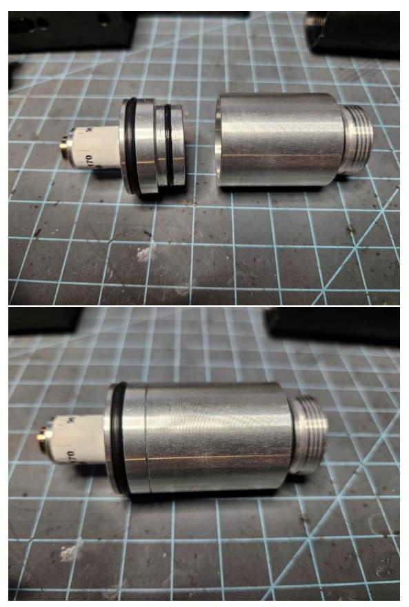
9) The regulator will need to vent to the atmosphere. Start by screwing the valve body back onto the air tube. Be sure it is tight. The vent location can be in any orientation you choose, however, it is easy to line it up on the bottom of the tube because the valve body set screws are located on the bottom of the valve body.
