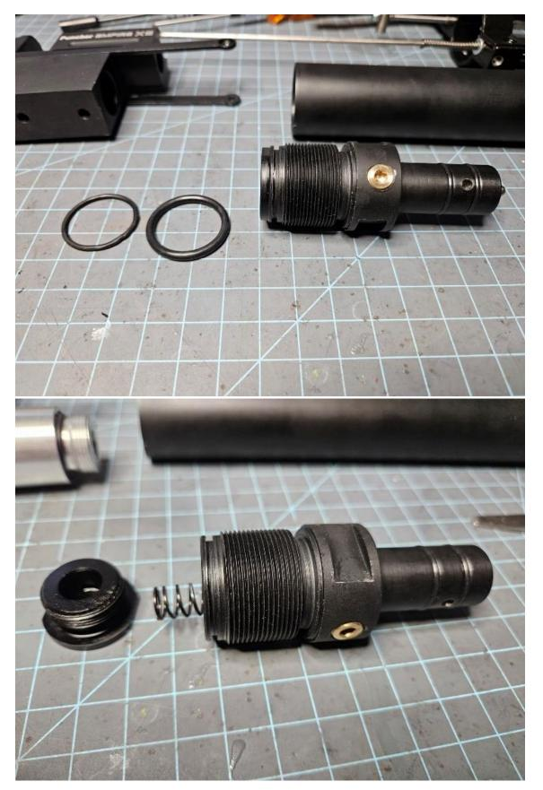
8) Lubricate the o-rings on the regulator. Then, push the regulator into the plenum.
