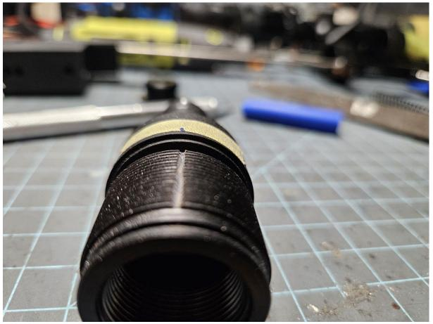
11) Using a triangular file or Dremel with a thin cutoff wheel, cut a small notch at the previously marked location. When, the valve body and air tube are reassembled, air will be able to no vent from the regulator, down the valve body channel, and out of the air tube notch.
