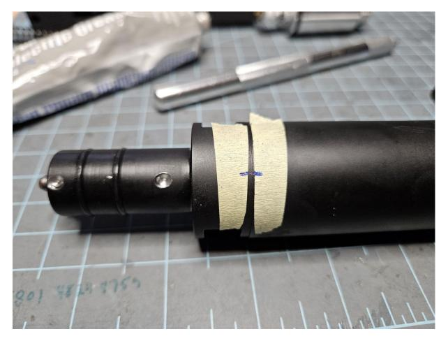
10) Using a triangular file or Dremel with a thin cutoff wheel, cut a channel inline with your mark into the threads of the valve body. Do not go any deeper than the bottom of the threads.
