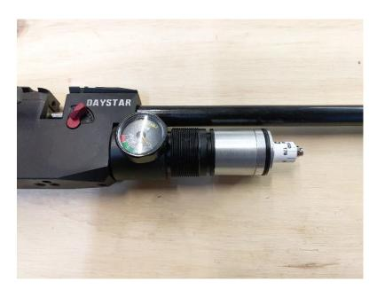
To improve regulator ventilation a groove may be filed in the thread of the body. This will not affect the gun when used without the regulator in the original configuration.
