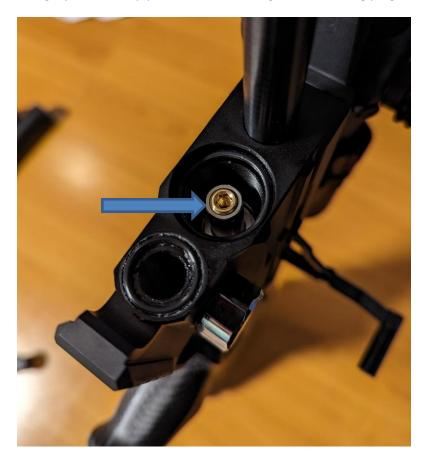
Using a pair of needle nose pliers, gently pull out the factory regulator.
