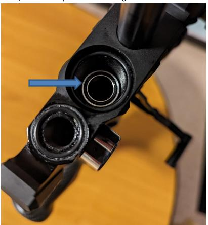
Set the Huma regulator to the desired pressure, then place the main regulator body in, like this...
