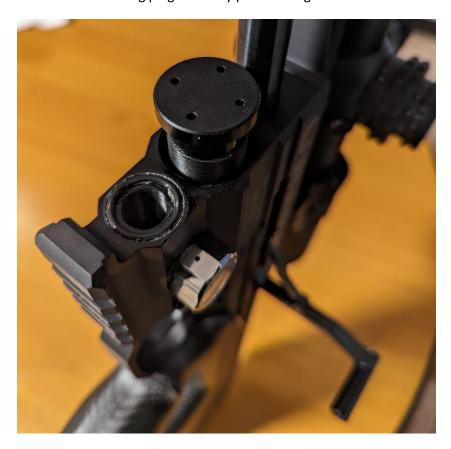
Finally tighten the retaining plug with the Circlip pliers, make sure the bleed grub screw is tight, reinstall the air bottle, making sure the O-ring is in place and lightly greased, and refill the air rifle!
